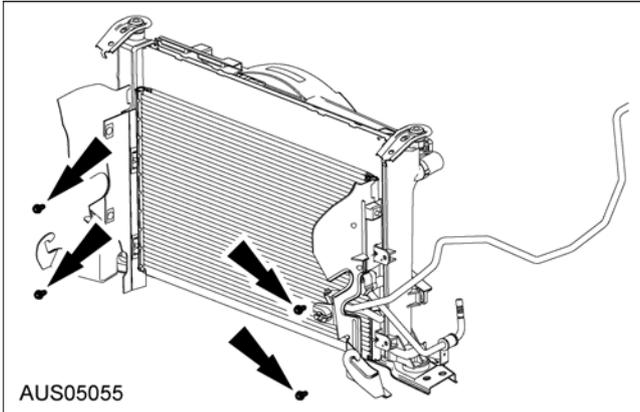
2. Remove M10 firtree attaching Radiator side shield 8110/1 to headlamp support panel on LH and RH side. 2 in total
