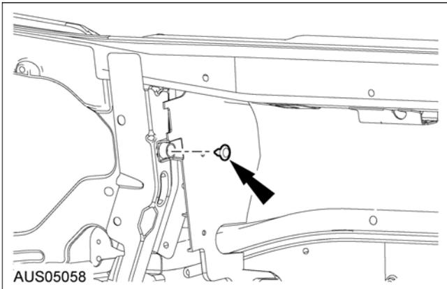
4. Remove screws connecting condenser to radiator on both LH and RH side. 4 in total
