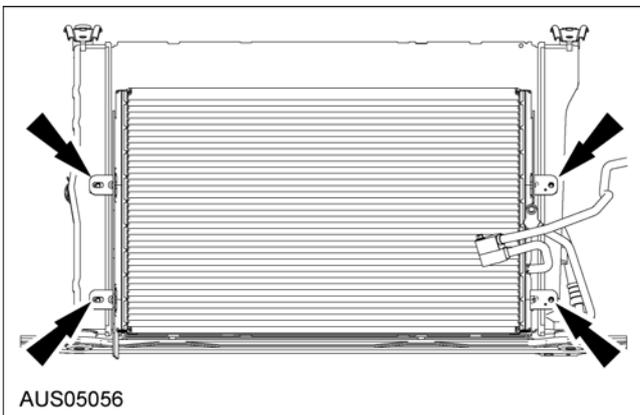
5. Remove Radiator side shield 8310/1 from condenser on both LH and RH side
