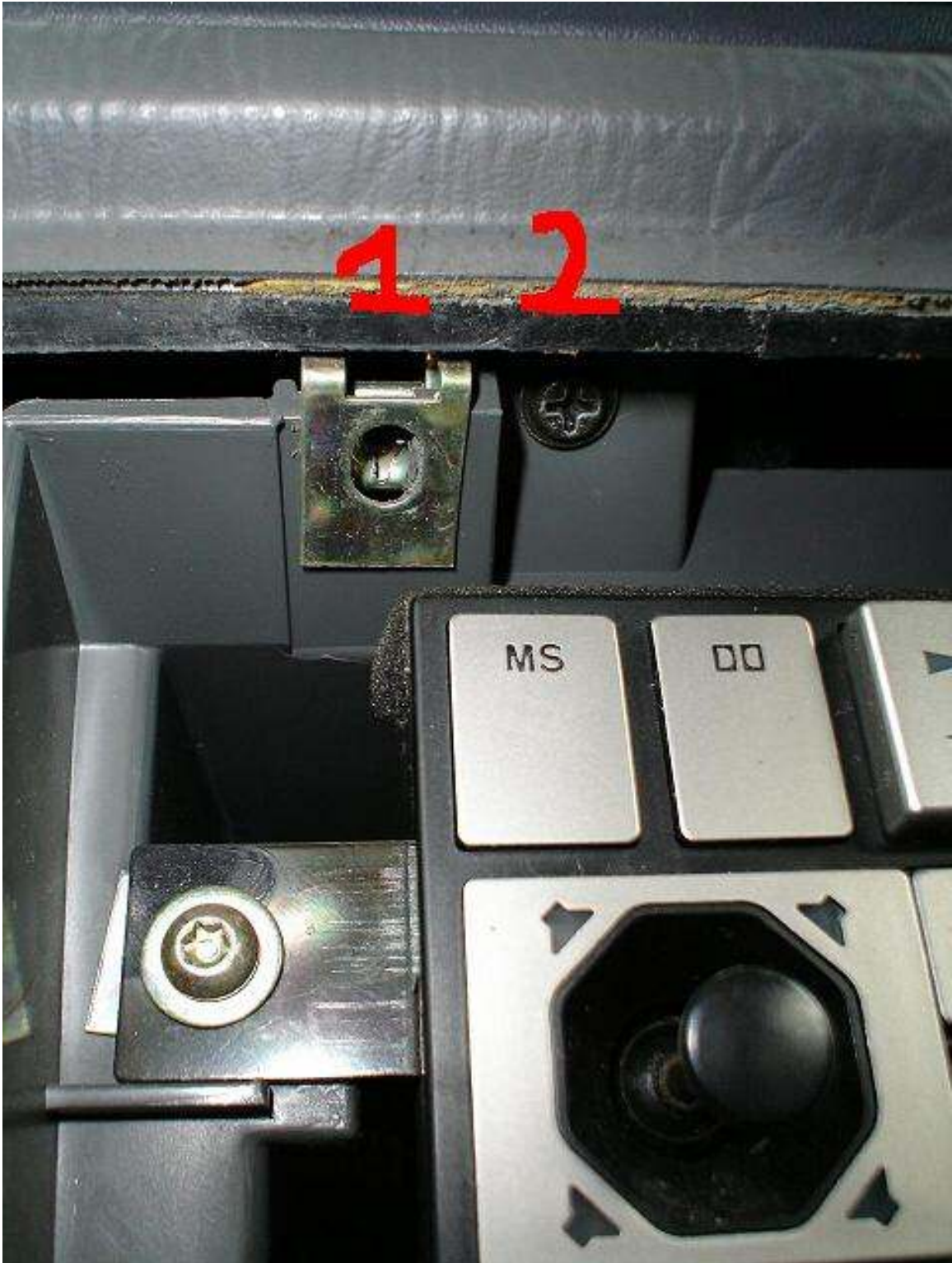
Screw locations on passenger side of head unit.
