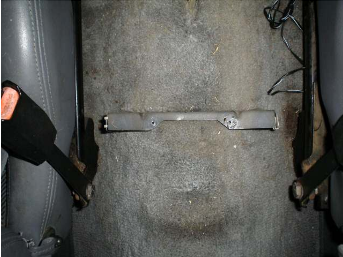
Centre console mounting point ("up" = towards dash).
