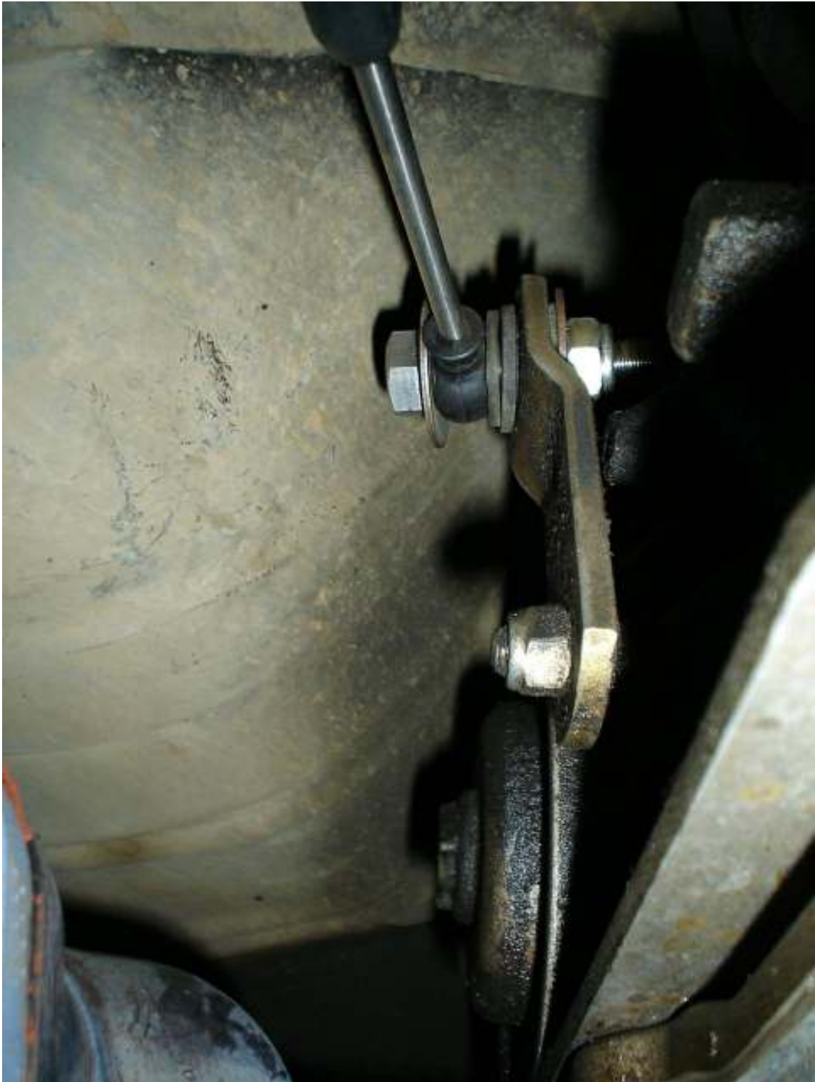
Cable meets shift point linkage. Note bolt & washers (there are only two washers, the other bits you see are from the grommet that sits in the end of the linkage).
