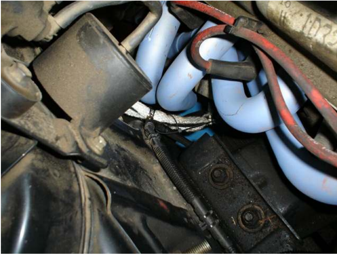
BA shifter cable looping around extractors (the engine has been cleaned since this disgraceful shot was taken!)
