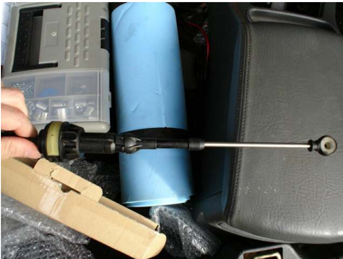
End of BA shifter cable (this end is attached to gearbox)
