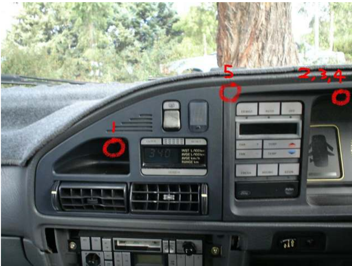
Screw locations for clock surround panel and instrument cluster surround panel.
