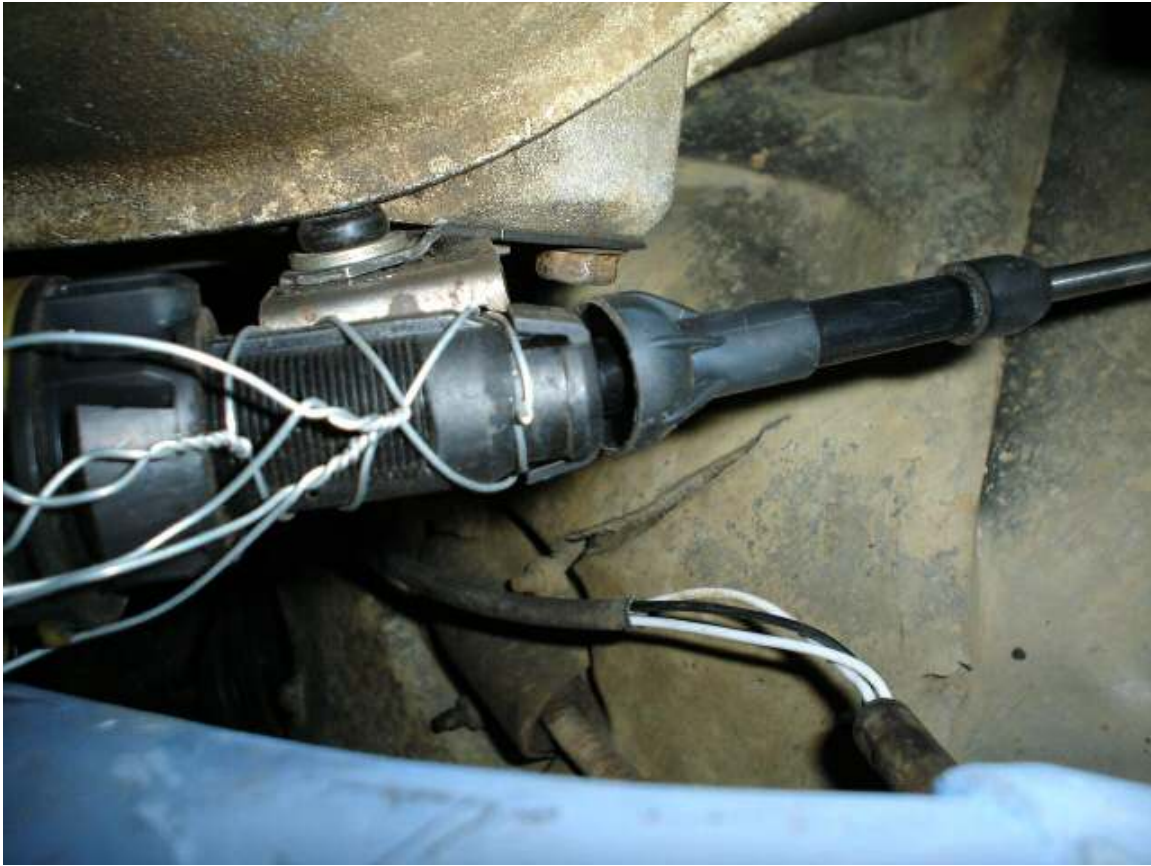
“Quality” fitting of cable to bracket using wire. The engine is to the left of this image (blue pipe = extractors).
