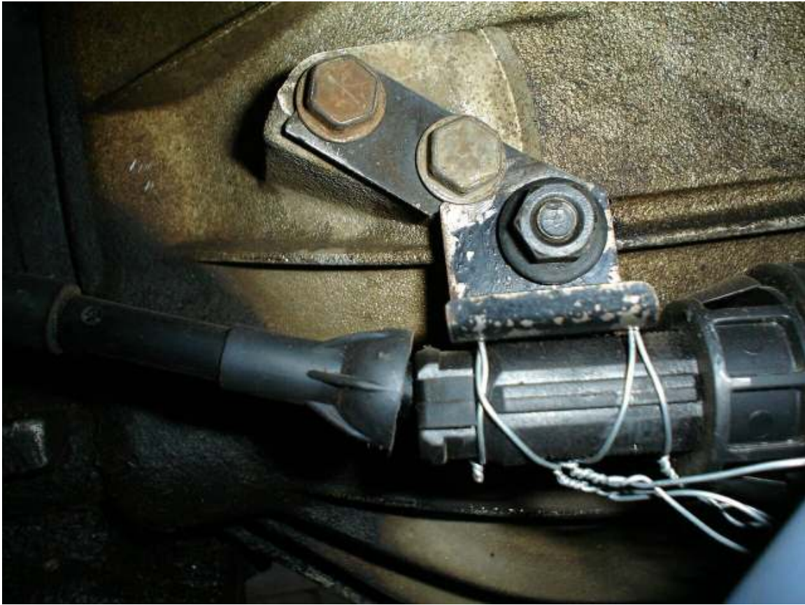
Bracket holding cable (from side-on).
