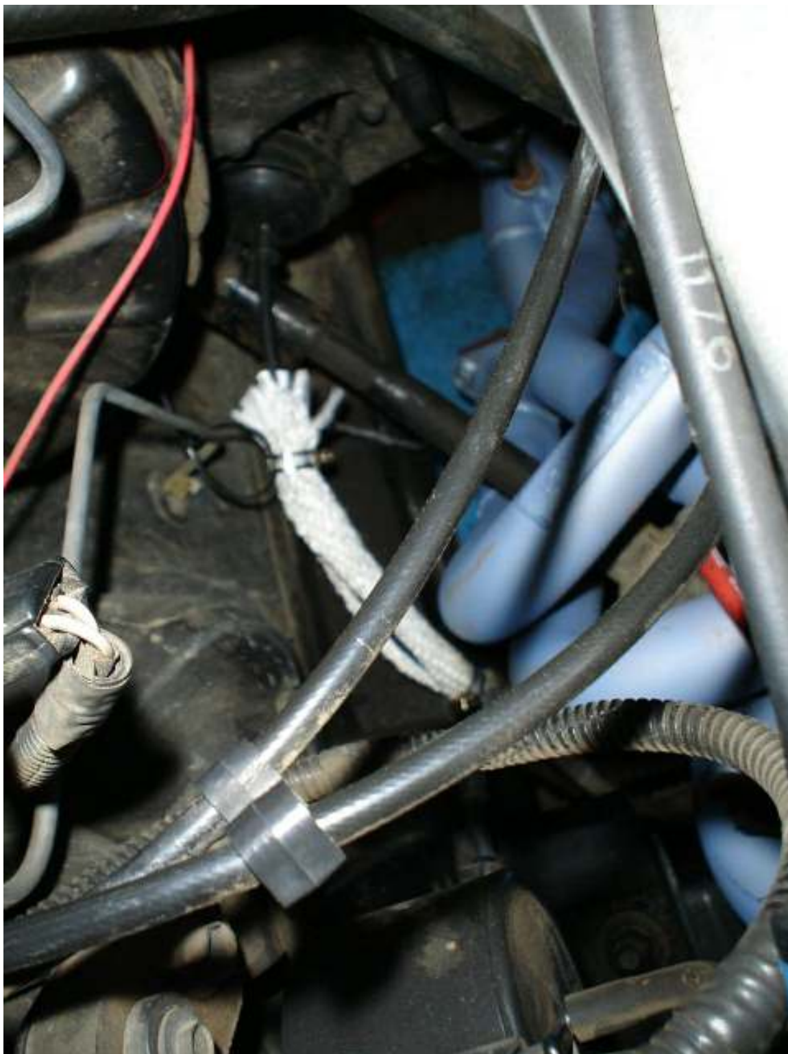
BA shifter cable (wrapped in heatproof bandage) coming from steering column plate.
