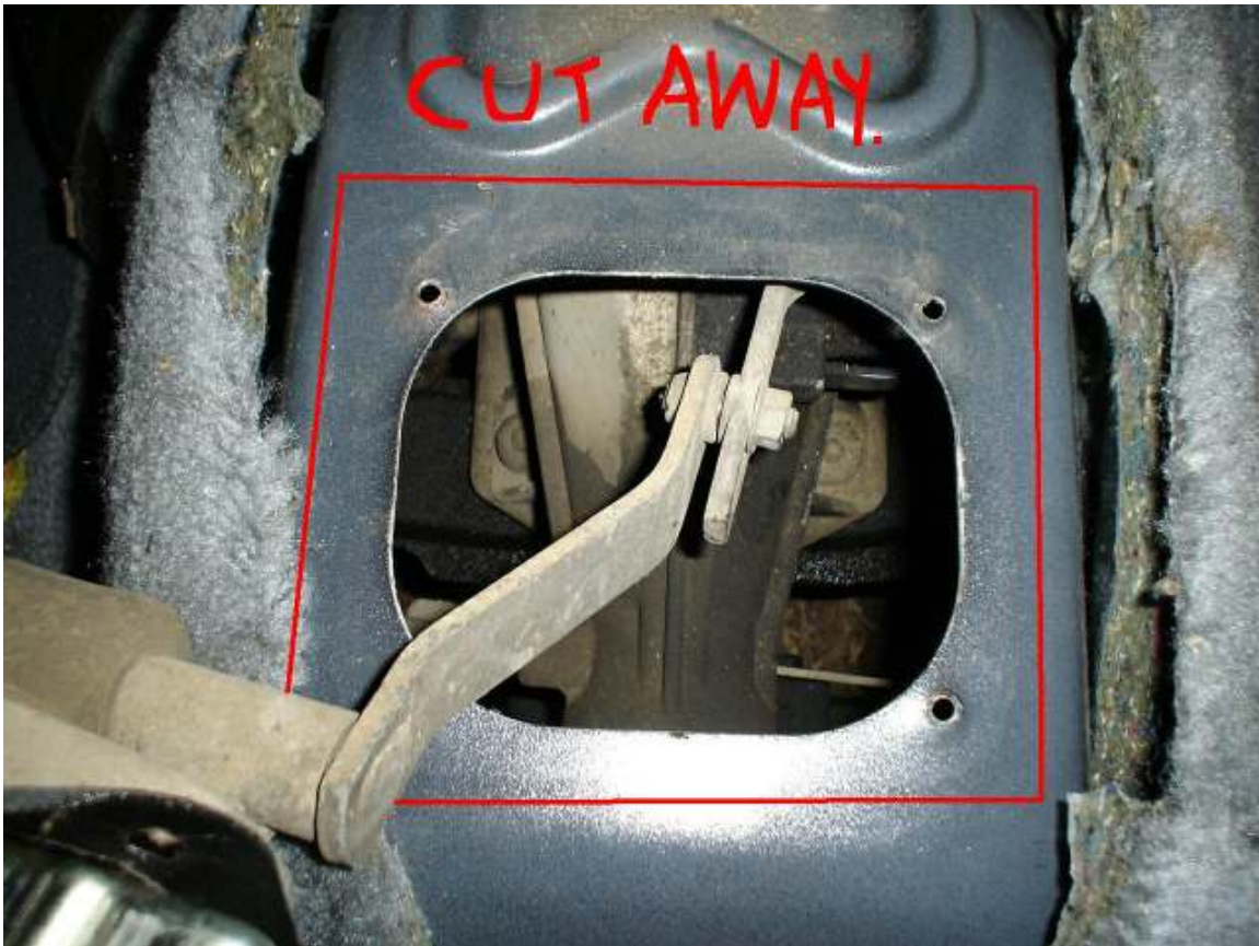
Removal of EB shifter and linkages
