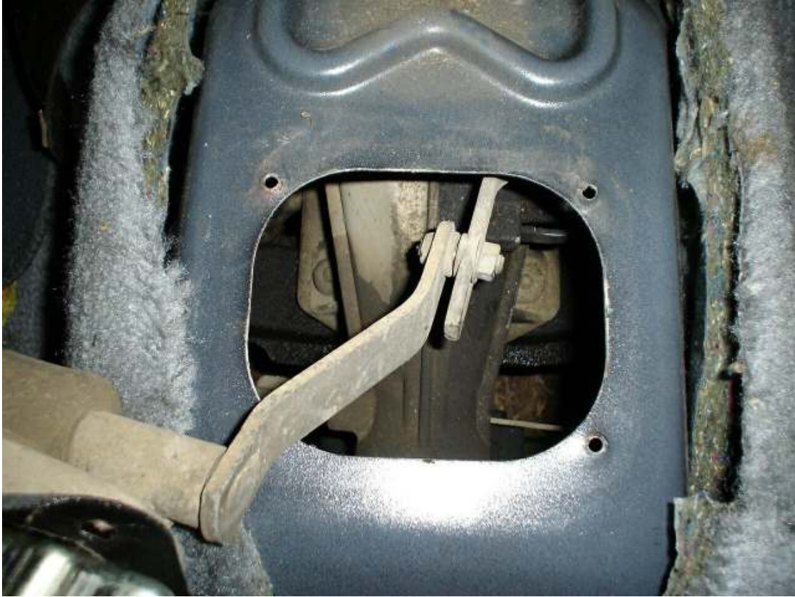
Removal of EB's shifter housing and linkages
