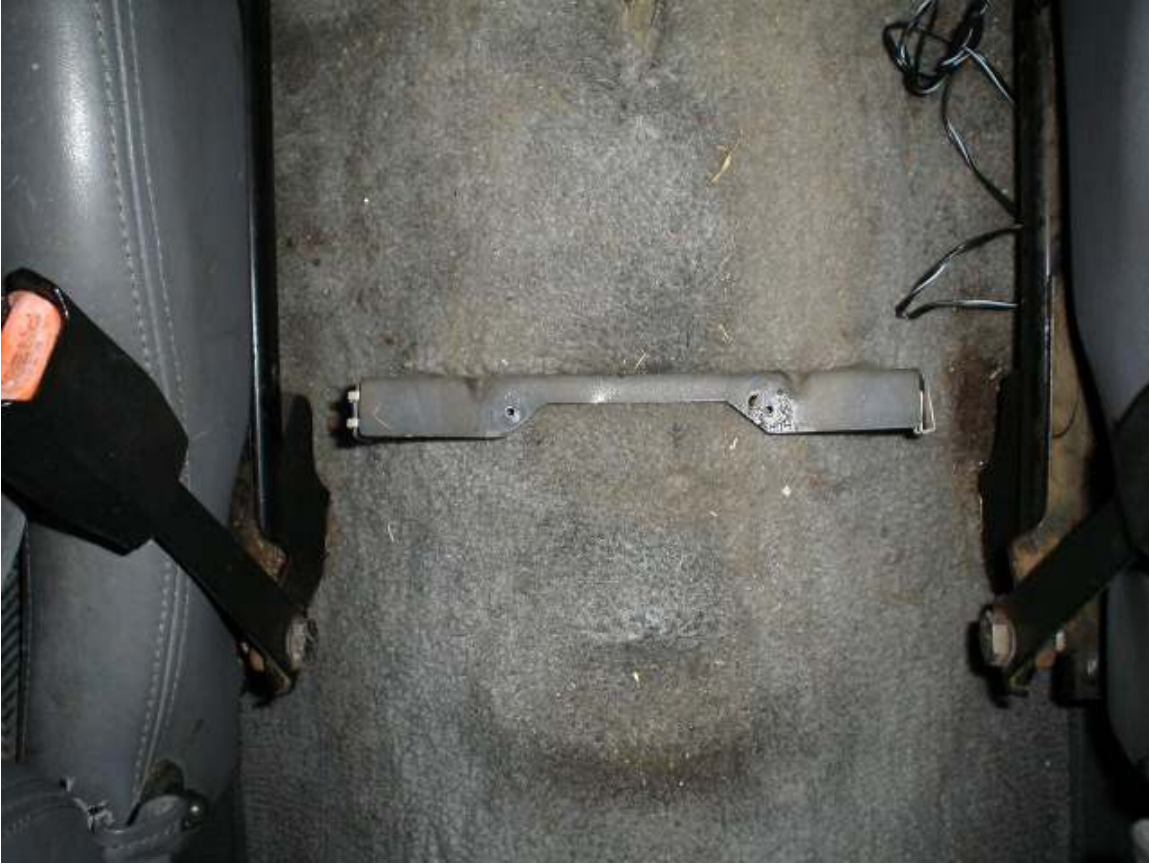
Centre console mounting point (“up” = towards dash).
