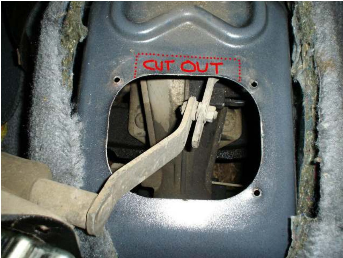
Removal of EB shifter & linkages.
