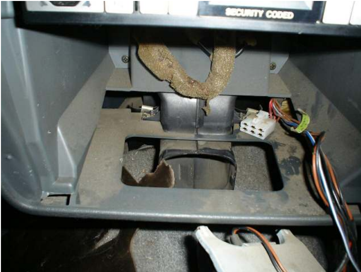
Power/Econ button loom (unplugged) and ciggy lighter loom. NOTE: the centre console has already been pulled out in this photo.
