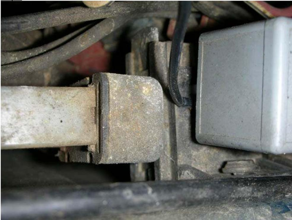
Now put the relay back in and have the wire running out the side. This will make the relay continue to operate as normal however our wire is now earthing out that pin the relay.
