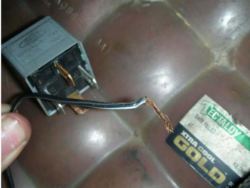
The next step is to bare the end of the wire and bend it at a right angle as you can see in the picture.
