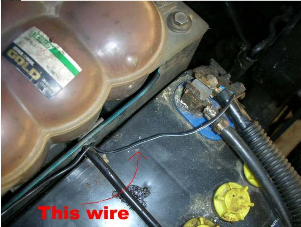
The first step is to attach a piece of wire to the negative battery terminal and the best way to do this is by crimping a ring styled crimp plug (pictured below) onto the end and bolting it on with everything else.
