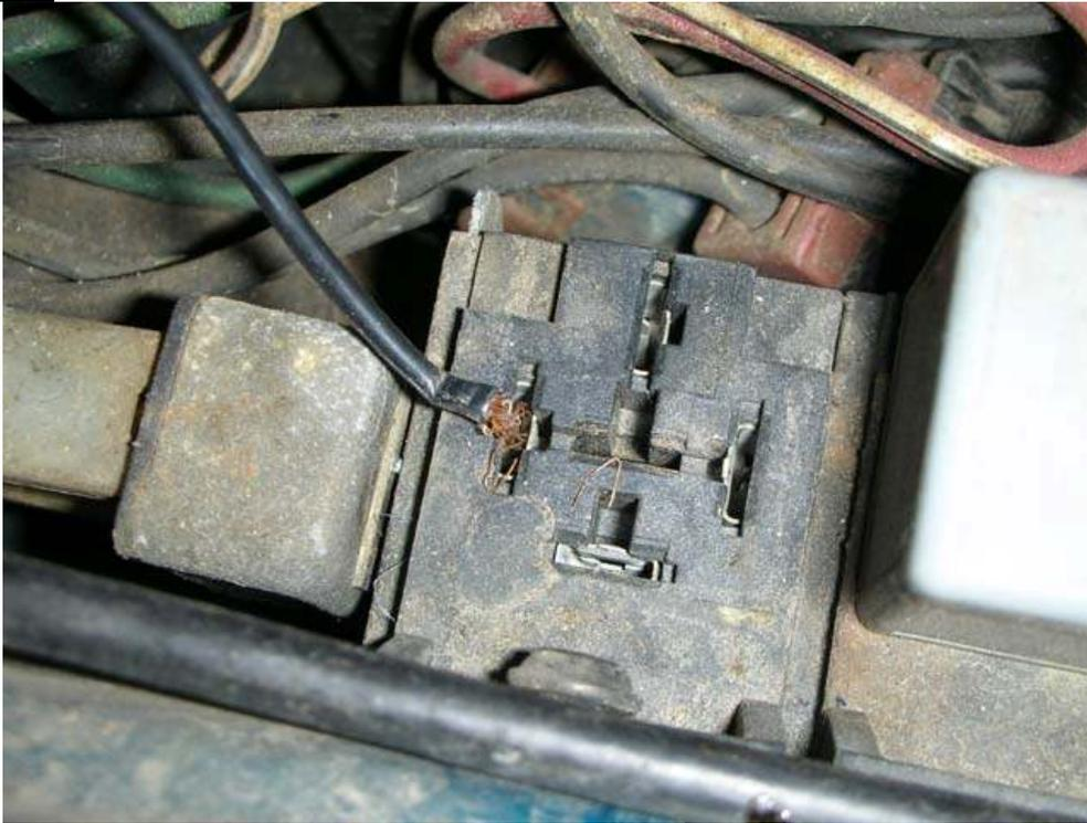
Now, pull the rear most relay out and stick the wire in the rear most slot (which is pin 85 or 86).
